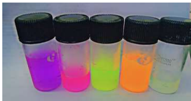
Figure 6: The fluorescence emitted by the Carbon Quantum Dots
