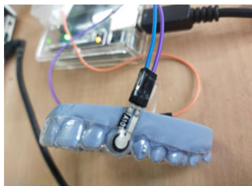
Figure 1: FSR402 sensor interfaced with an Arduino Uno
