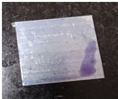
Figure 1: Dip-coated aluminium substrate
