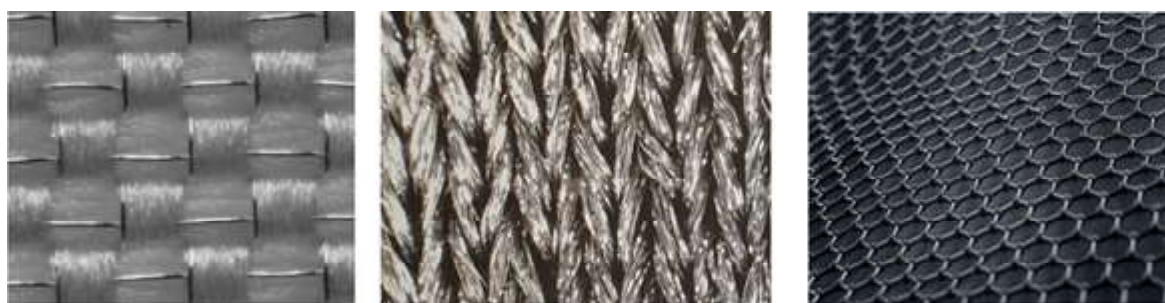
Figure 2(a): Woven conductive fabric with copper and nickel plated Nylon (b) Knit Jersey conductive fabric with cotton, silver, yarn and spandex (c) conductive graphene sheet
