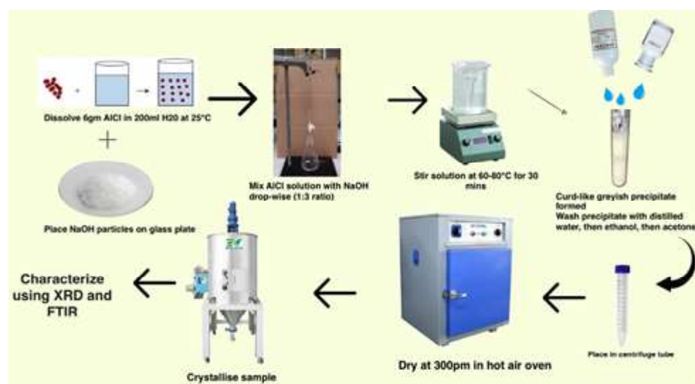
Figure 1: The process of synthesizing the required AlO nanoparticle
