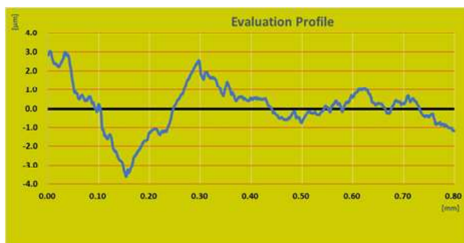
Figure 5: Surface roughness evaluation profile of the dental composite incorporating AlO nanoparticles
